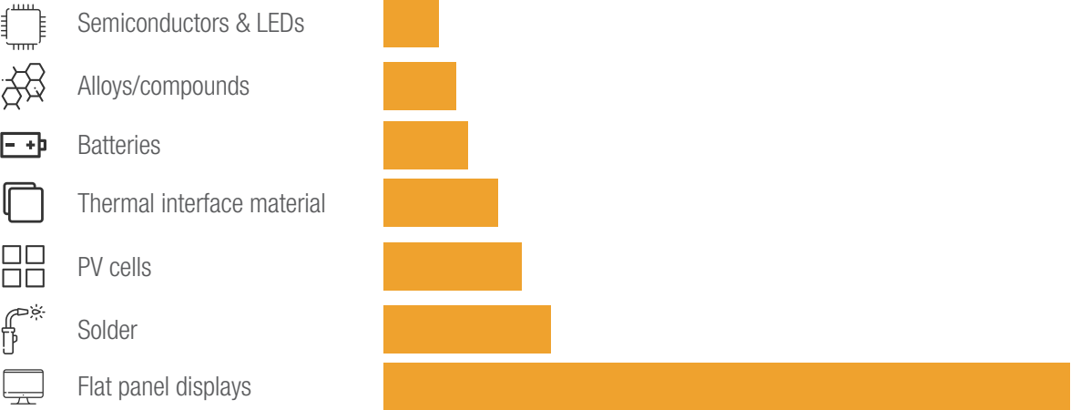
Figure 13: Applications of indium (European Commission, 2020; based on NACE2 sectors assignment; own elaboration).
